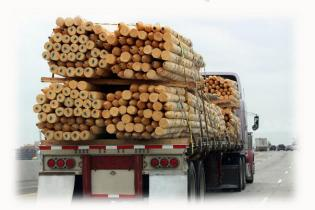
**CREOSOTE:** Pressure treated per AWPA Standards / Min 8# per cubic foot retention **CCA:** Pressure treated per AWPA Standards / Min .40# per cubic foot retention
